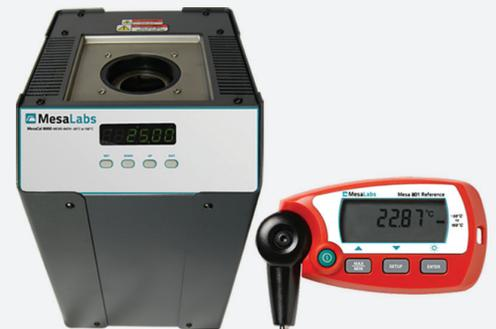
*Mesa Lab’s MicroBath and Reference Thermometer products used for industrial temperature calibration*
