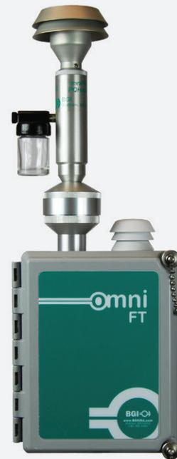
*Mesa Lab's Omni FT provides a flexible, low cost solution for EPA air pollutant monitoring studies*
